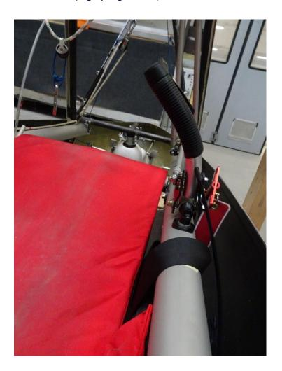
Double pedals – wheels and winglets - rudder (conventional sense!) .
